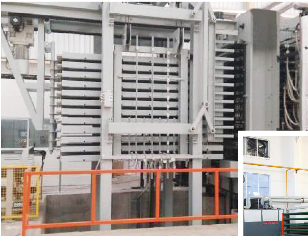
Capacity: 80 – 150 sheets/h Opening No: 10–15 layers
