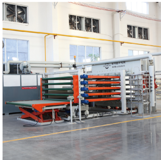
Capacity: 60 – 80 sheets/h Opening No: 5–6 layers
